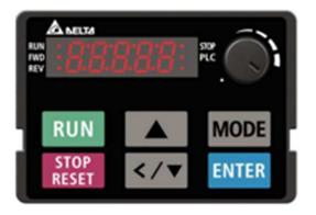
Normal display (home screen) on the Delta VFD can be rotated between the displays listed below, by using the **MODE** button.
